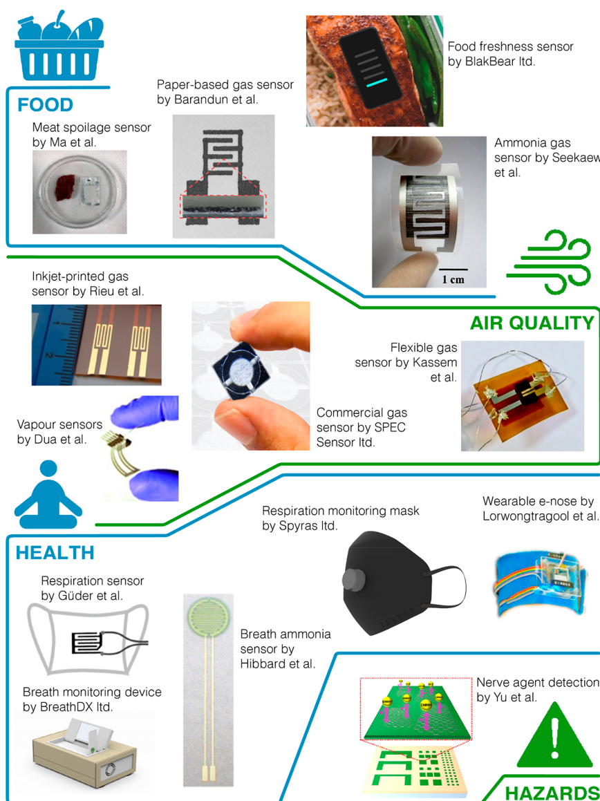
Figure 4. Printed gas sensors in different areas of application. Panel food (from left to right): Reprinted in part with permission from ref 154. Copyright 2018 American Chemical Society; Reprinted in part with permission from ref 55. Copyright 2019 American Chemical Society; Reprinted in part with permission from BlakBear Ltd. Copyright 2022 BlakBear; Reprinted with permission from ref 80. Copyright 2014 Elsevier. Panel air quality: Reprinted with permission from ref 175. Copyright 2016 Elsevier; Reprinted with permission from ref 120. Copyright 2010 John Wiley and Sons; Reprinted in part with permission from SPEC Sensors Ltd. Copyright 2022 SPEC Sensors; Reprinted with permission from ref 61. Copyright 2013 Royal Society of Chemistry; Panel health: Reprinted in part with permission from ref 201. Copyright 2016 John Wiley and Sons; Reprinted with permission from BreathDX Ltd. Copyright 2022 BreathDX; Reprinted with permission from ref 72. Copyright 2013 American Chemical Society; Reprinted with permission from Spyras Ltd. Copyright 2021 Spyras; Reprinted in part with permission from ref 197. Copyright 2014 MDPI; Panel hazards: Reprinted in part with permission from ref 204. Copyright 2019 American Chemical Society.
